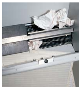
Automatic mechanical feeding system with revolving flaps
